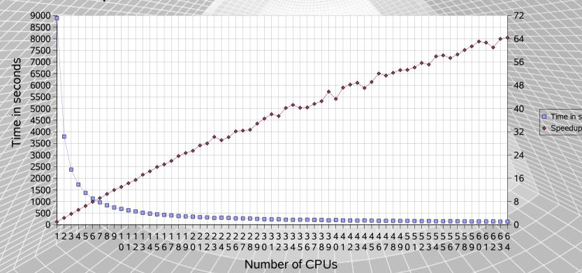
Simple numeric benchmark on a Sun Microsystems Enterprise 10000 with 64 UltraSPARC II CPUs
