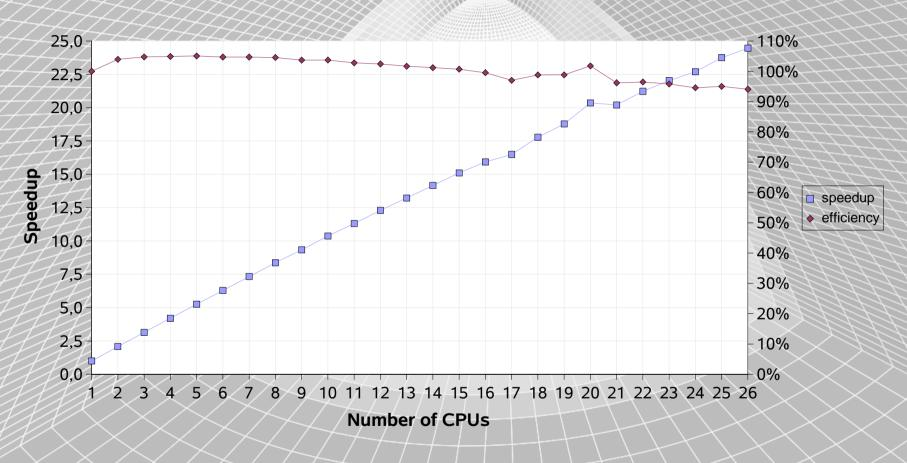
Results a 100 x 100 matrix doing 10,000 iterations with 400 threads on the E6000 (26 CPUs)
