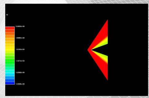
As a reference sample to check the correct communication (boundary update) of the JUSTGrid we computed a 3D cone with the JUST Euler 3D solver and CFD++
